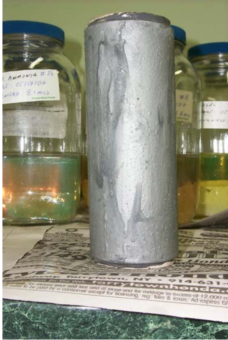
Sample #25 Exposed to 5% Ammonia
